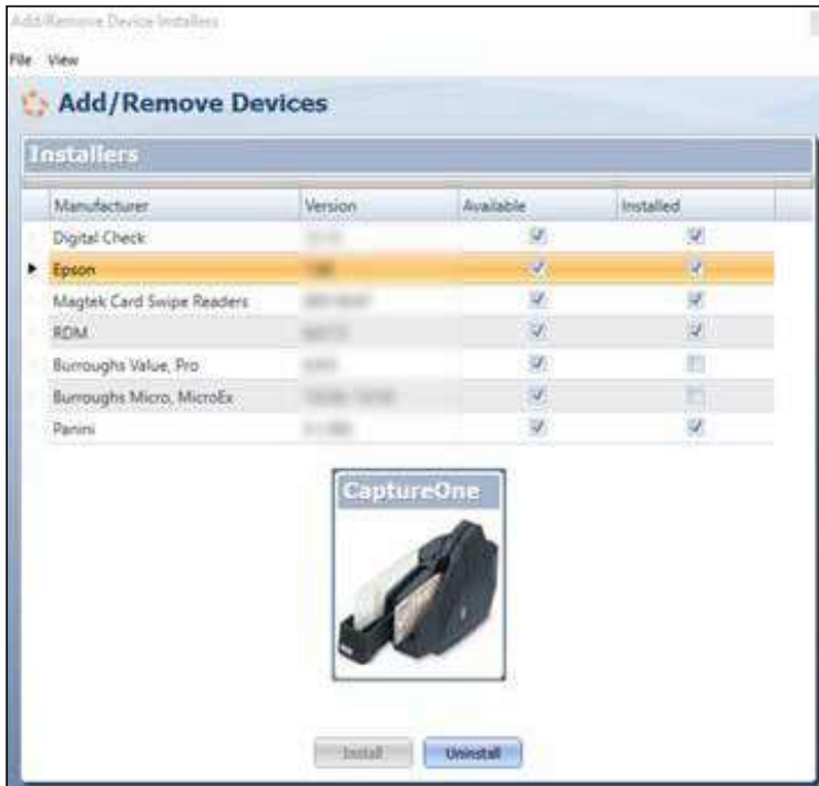
FIGURE 20 - SELECTING A SCANNER WITH UNINSTALL OPTION
