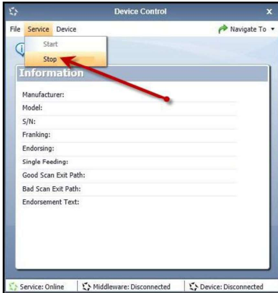
FIGURE 15 - STOP DEVICE CONTROL SERVICE
